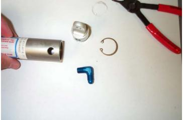
Install an AS568A-212 O-ring onto the new actuator end P/N 9-33106-01 or -02.
