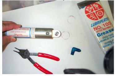
Coat the 90 degree fitting threads with thread compound Loctite<sup>™</sup> 565) then reinstall the fitting to approximately the angle shown.
