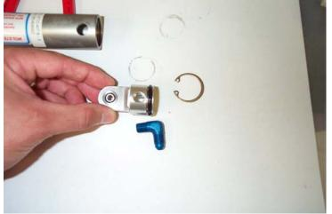
Grease the O-ring using Mil-H-5606 hydraulic fluid, Lubriplate No. 105, or similar.
