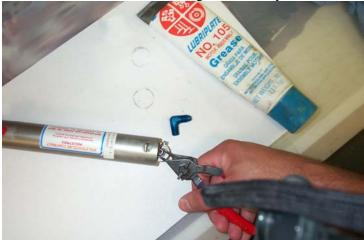
Pull the actuator end out line up the hole in the cylinder with the hole in the actuator end.
