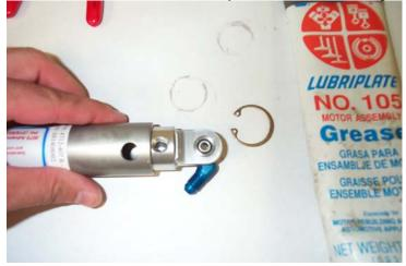
Push the actuator end far enough into the cylinder that the snap ring can be installed.
