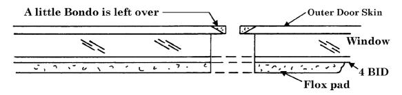
Step 4) Drill out the hole with the counter bore (#08860108) bit. As you approach the carbon with your bit, slow down and carefully watch for black shavings. As <u>soon</u> as you see black, stop drilling. Inspect the bottom of the hole carefully with a flashlight, you must drill completely through the window, <u>removing as little of the carbon skin as possible.</u>
