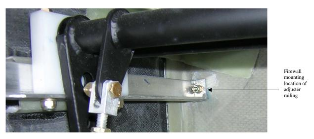
Figure 12.3.E.5 Standoff attachment to fuselage using carbon layups
