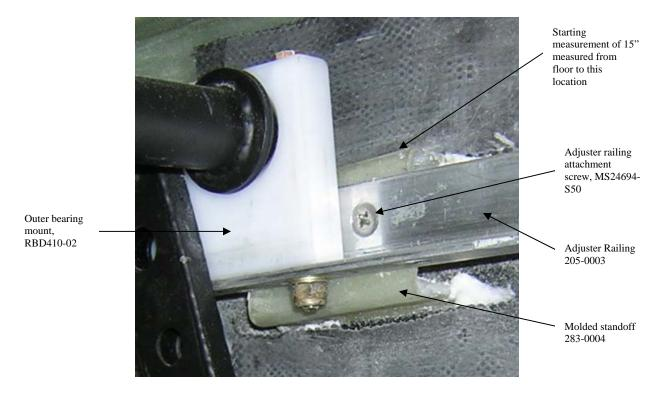
Figure 12.3.E.4 Railing attached to Firewall
