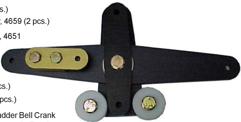
Completed Rudder Bellcrank Fig. 17:G:1a
