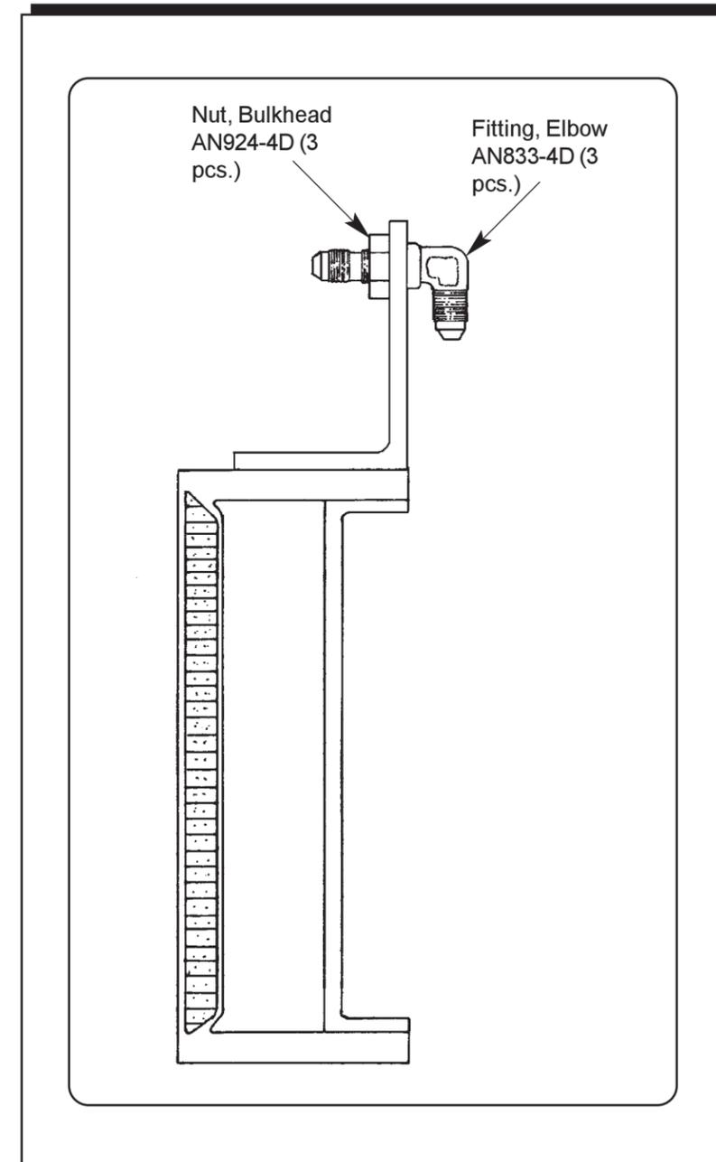
**Hydraulics: Lines Going to Hydraulic Valve**
