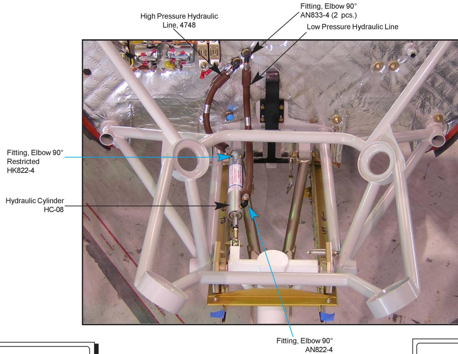
**Note:** Restricted fitting should be installed on the high-pressure side of the cylinder.
