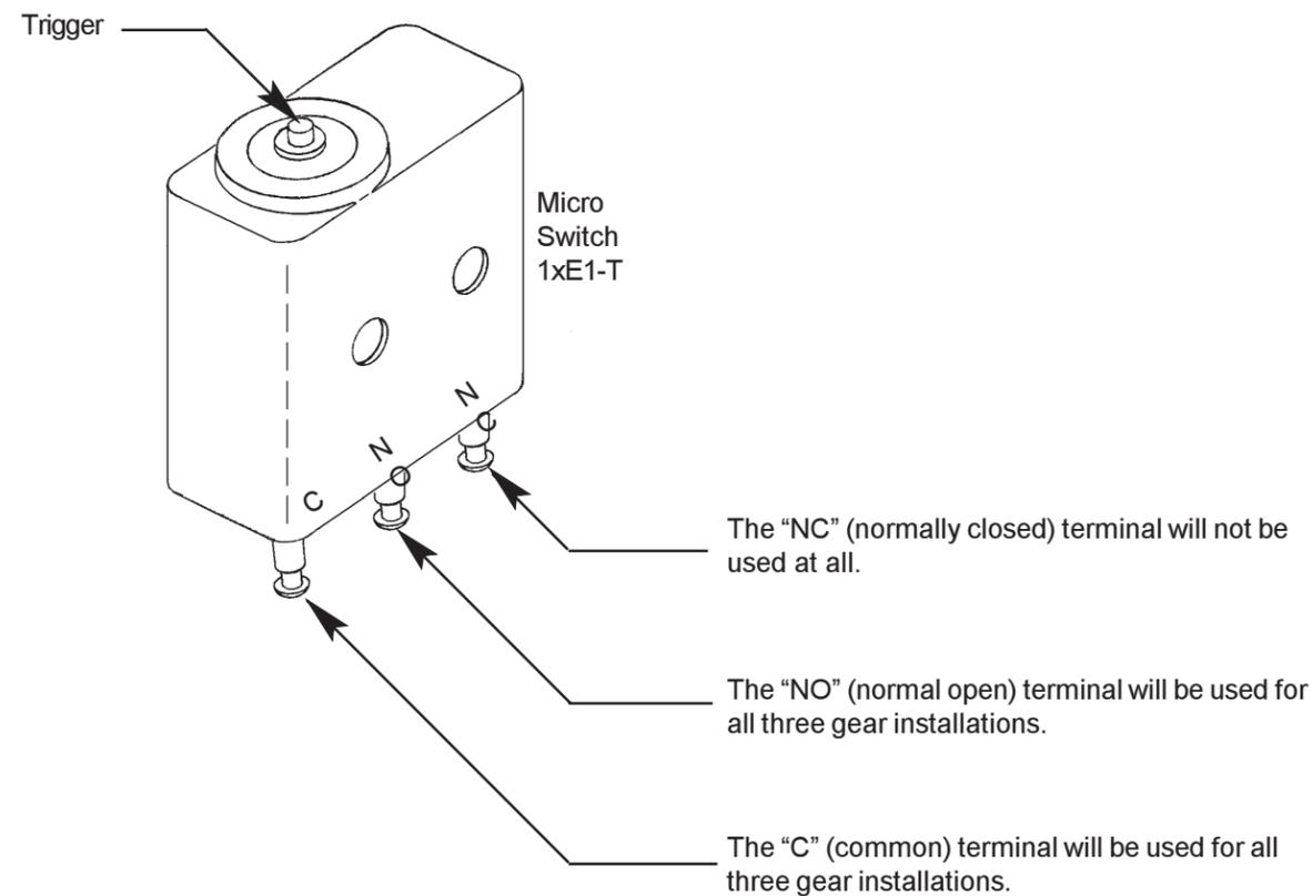
The micro switch wires should be soldered directly to the switch.
