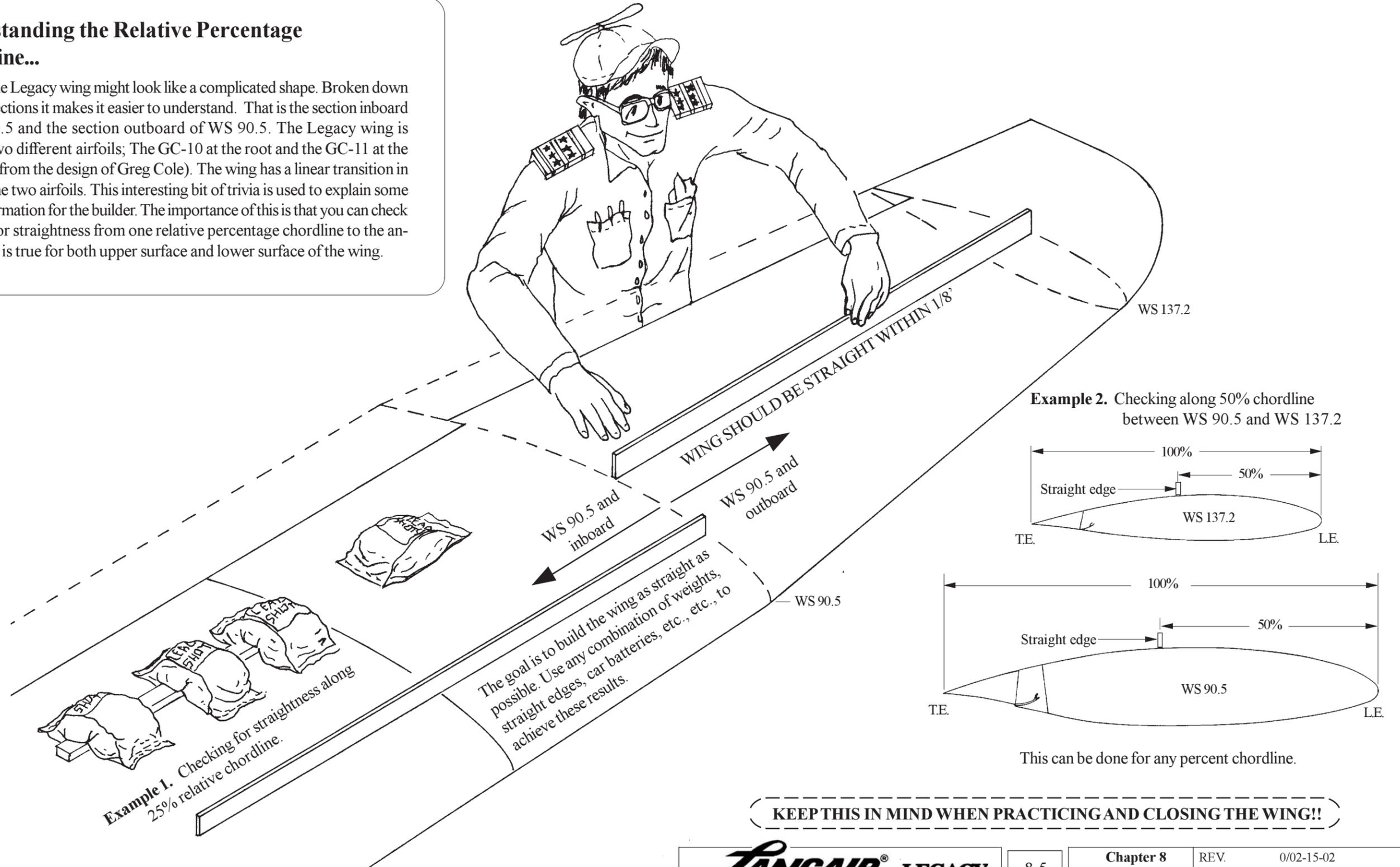
**Example 1.** Checking for straightness along 25% relative chordline.
