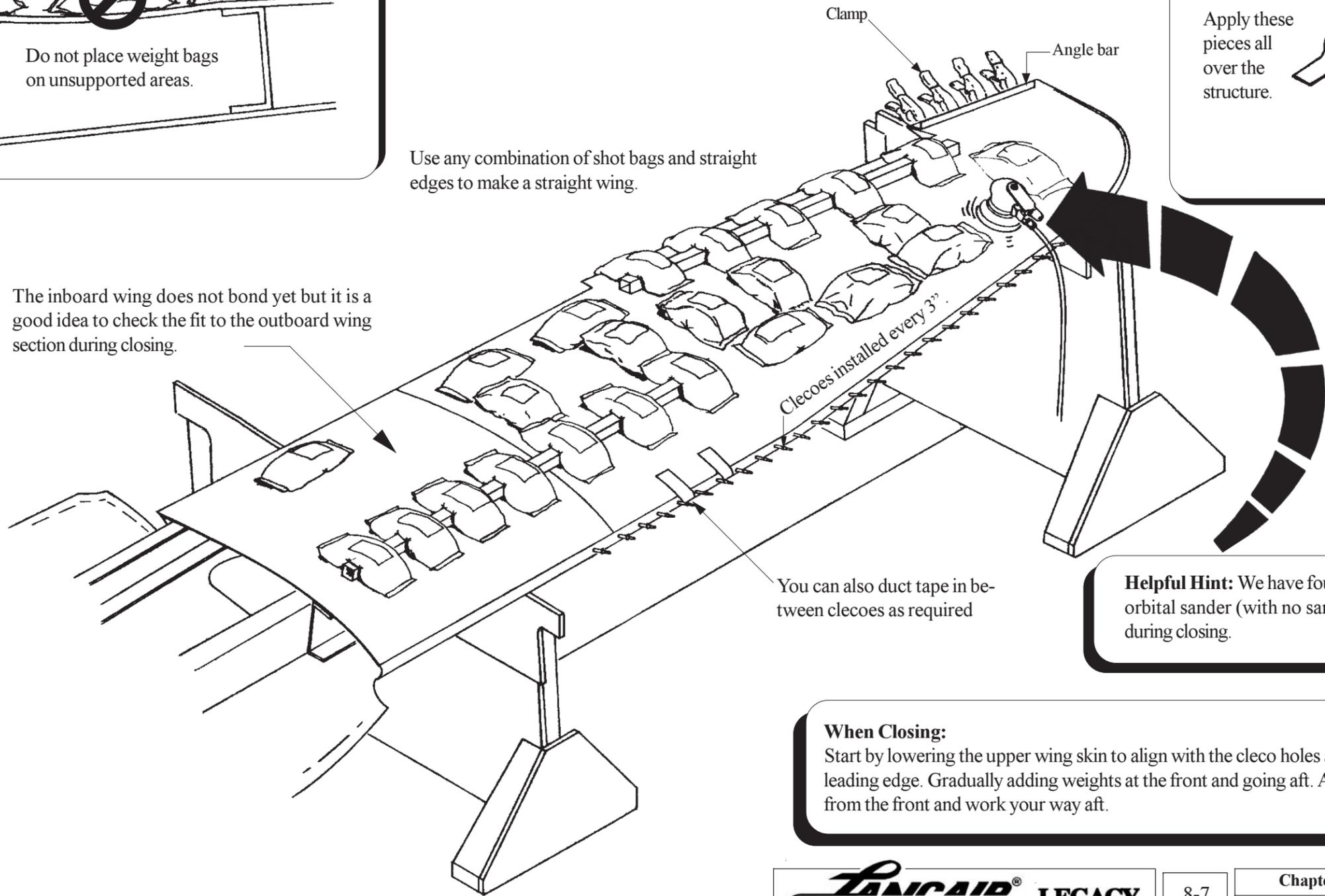
**Helpful Hint:** We have found that using a padded dual action orbital sander (with no sand paper) helps settle the adhesive during closing.
