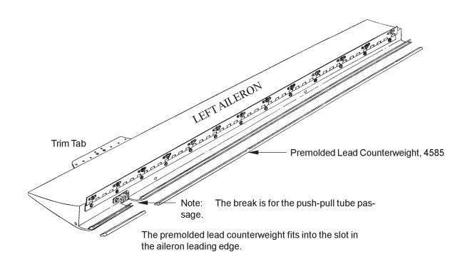
Suggestion: Use a pointer as a reference for balancing (You can't leave the level on the aileron when checking the balance.)
