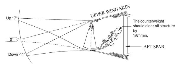
C 6. Install the aileron and check for proper clearance through the travel range.
