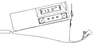
Note: The above figure shows the aileron 100% mass balanced at the wing tip.
