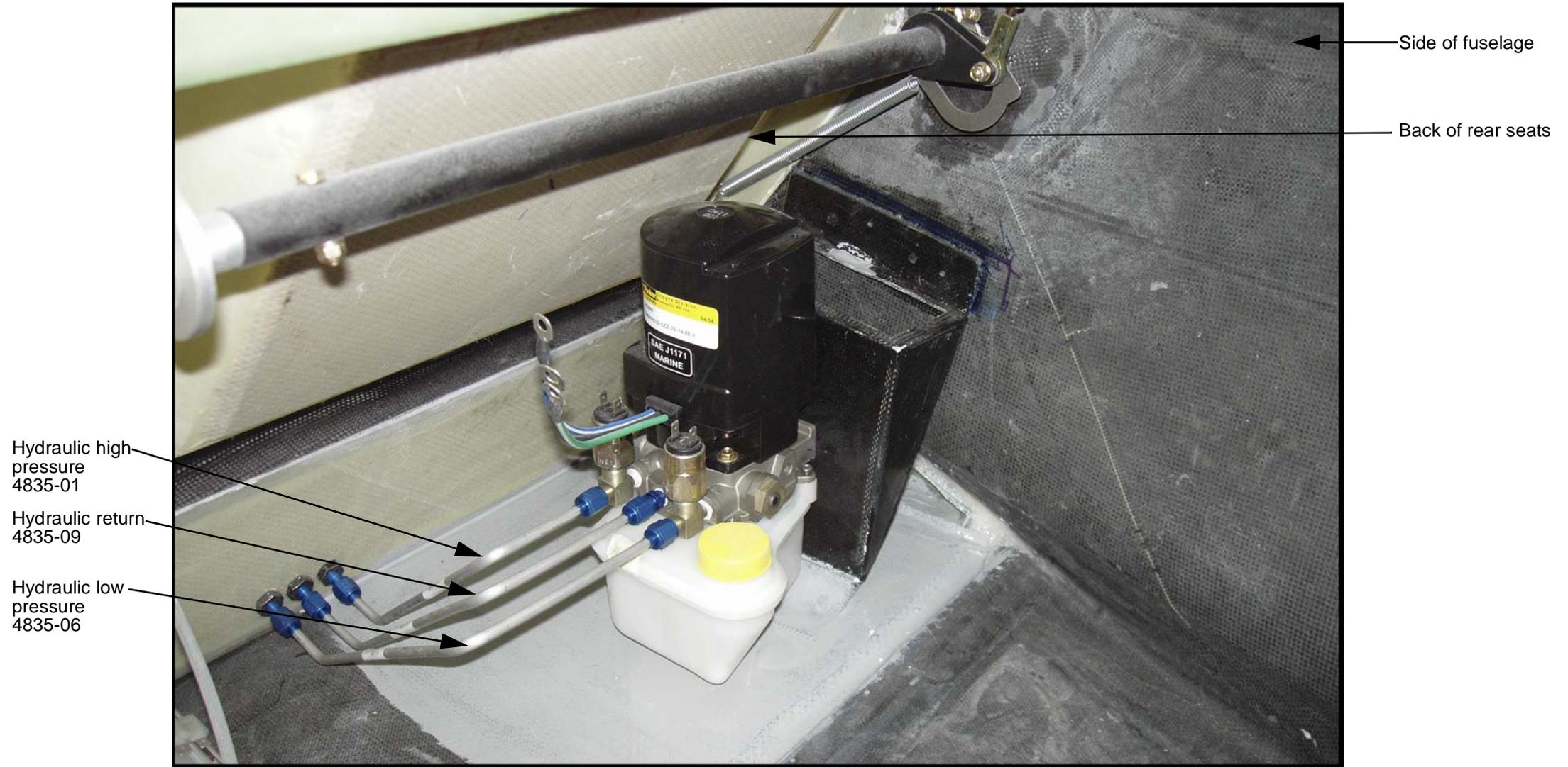
Figure S.2.0.5 Fuselage lines – view 2
