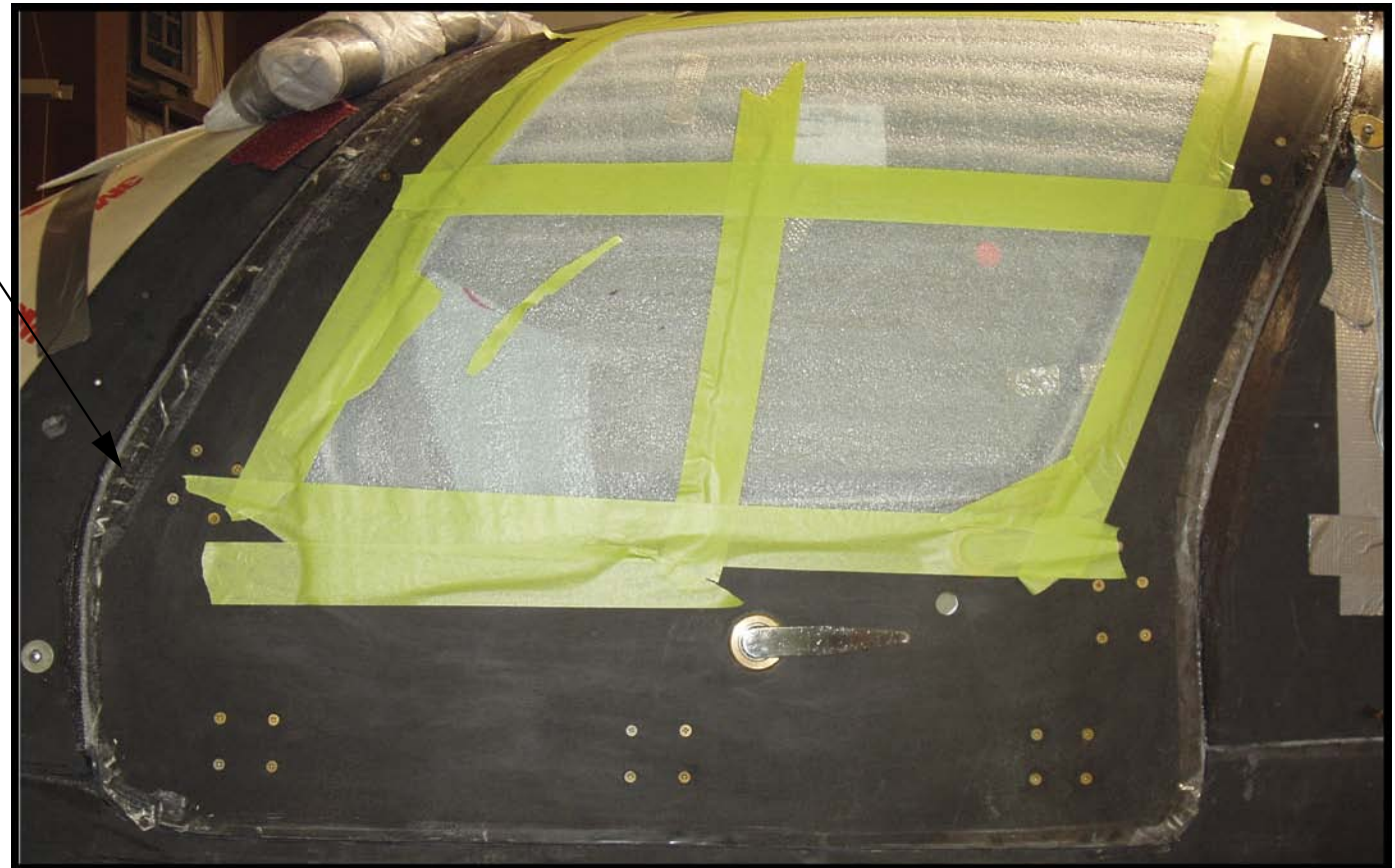
Figure S.2.C.1 Doorframe bonded to the fuselage
