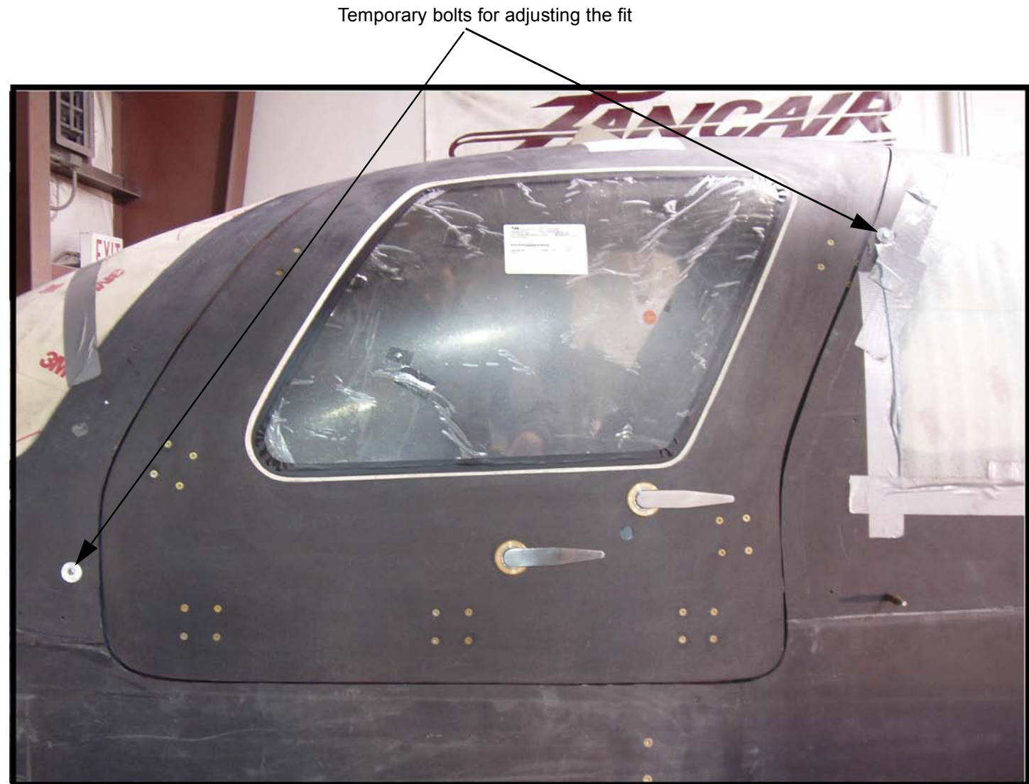
Figure S.2.B.2 Door reattached to the doorframe and fitting is in process
