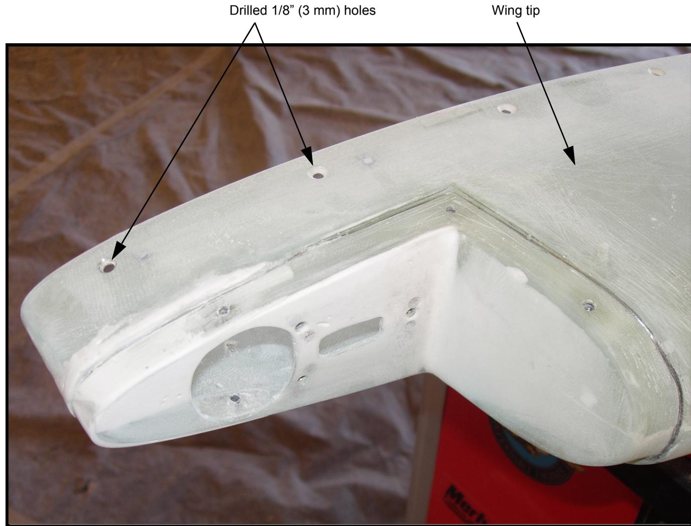
10. Make sure the wing tip rests against the flange in the L.E. area.
