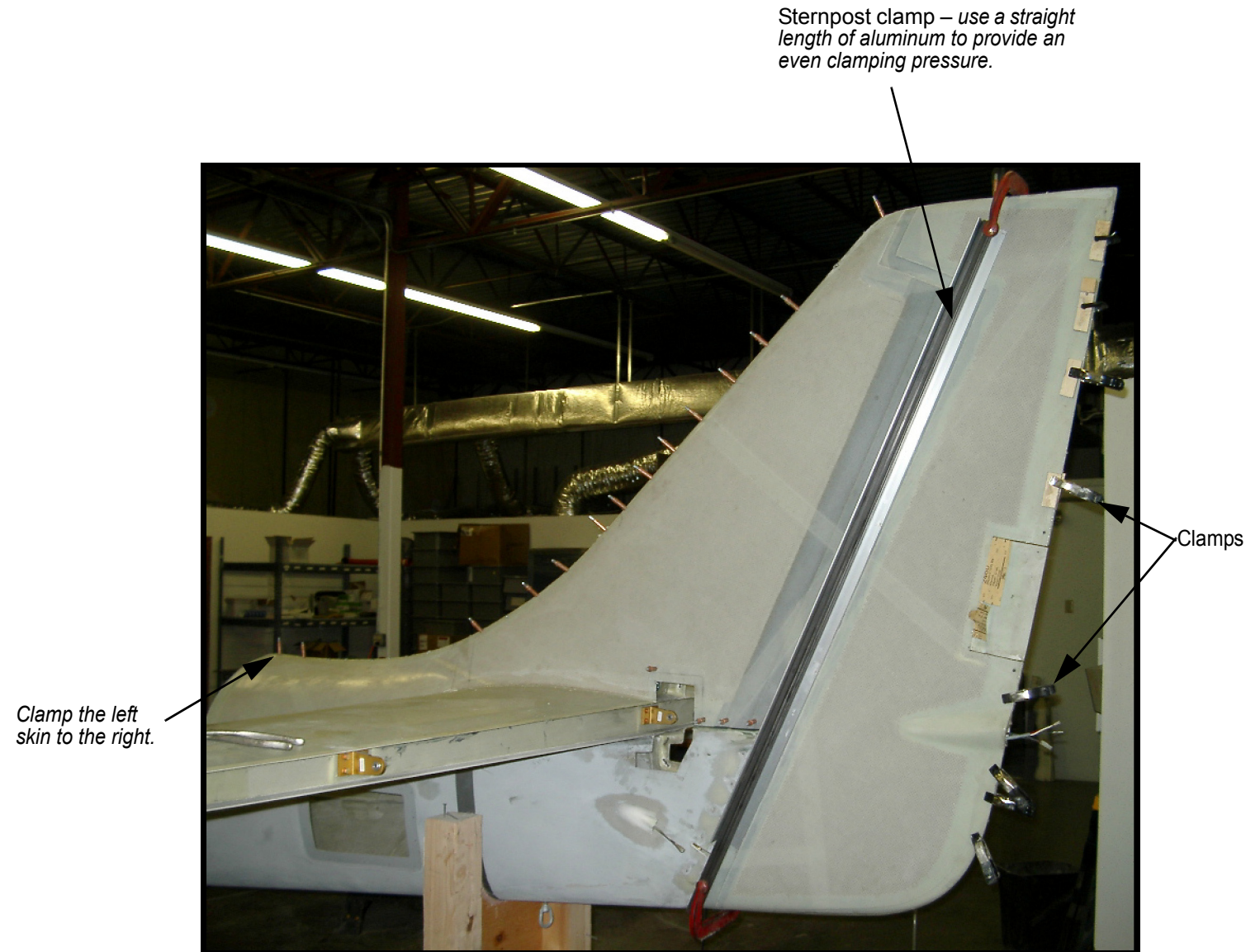
Figure 18.3.I.1 Clamping the left vertical stabilizer/rudder skin
