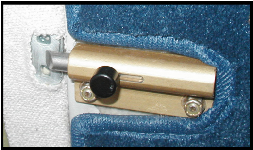
Figure 15.3.K.3 Completed aft seat latch
