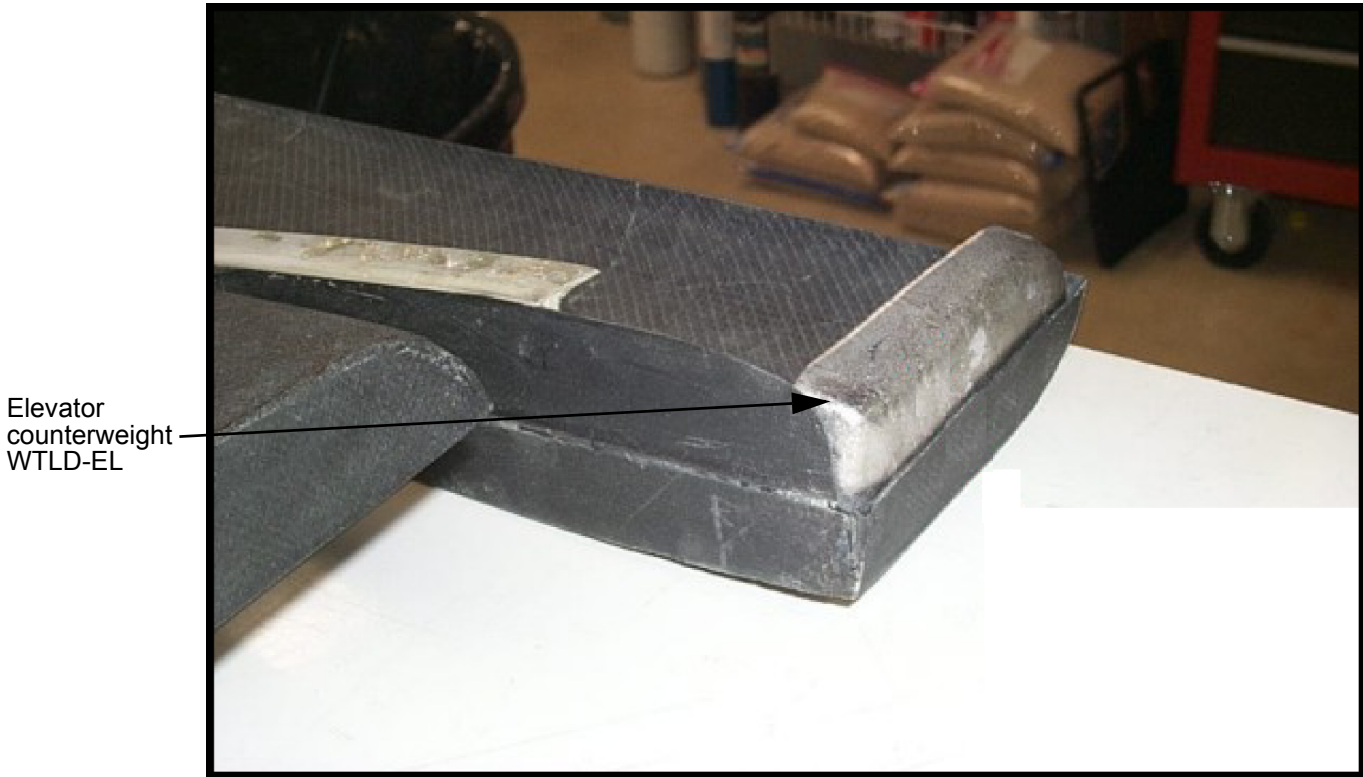
Figure 3.3.A.2 View of counterweight in elevator arm
