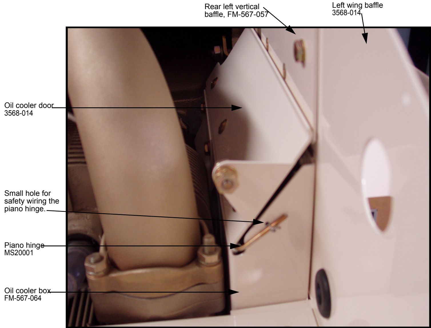
Figure 21.3.C.7 Oil cooler door and box installed with baffling
